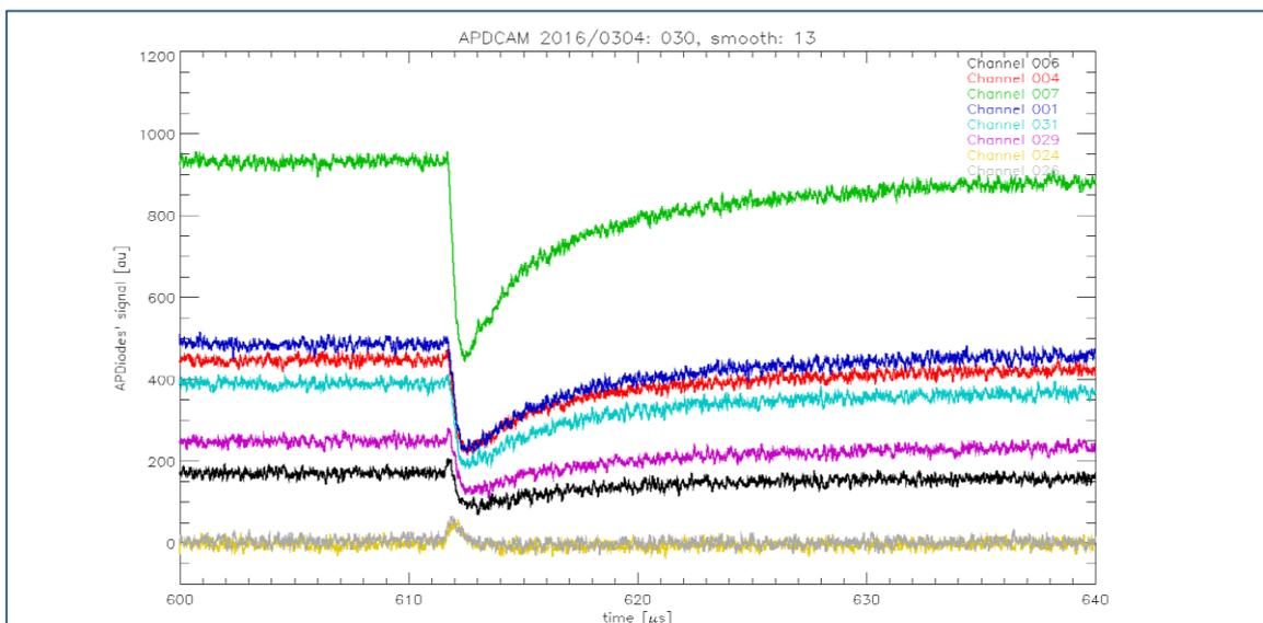
Figure 3. Time traces of the probing laser light in APDCAM. The estimated maximum light level is about  $10^{10}$  photons/s.
